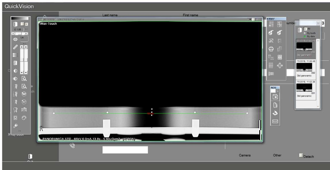
7. Measure also the two half of the image in order to check symmetry. The difference has to be max. 2mm.
