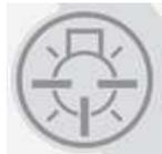
The key "Luminous centering device" helps turn ON/OFF the laser centering devices that allow the correct positioning of the medial-sagittal and Frankfurt planes, by adapting the I-Max Touch to the patient's anatomy.
