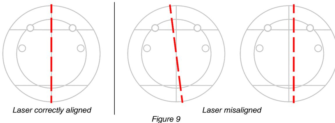
In case the test fails, repeat it checking that there is no mechanical interference. If misalignment is still present, call technical assistance.
